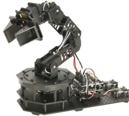
Fig: 1: Audrino based Robotic Arm
